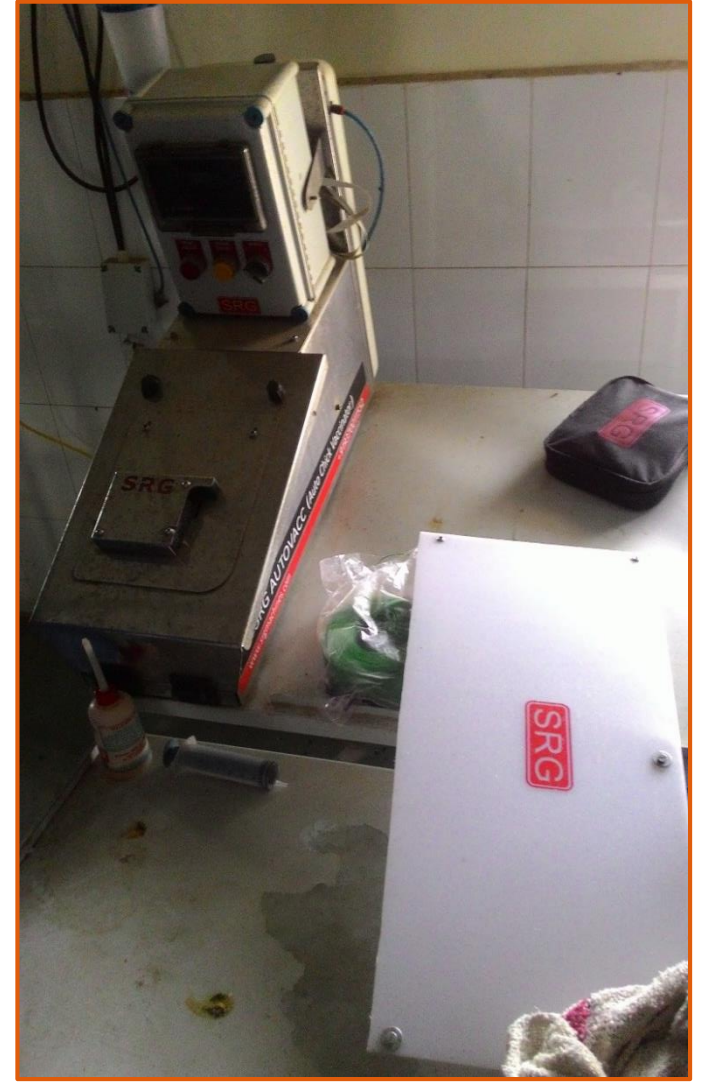
Automatic vaccination machine to vaccinate 50 chicks at a time
